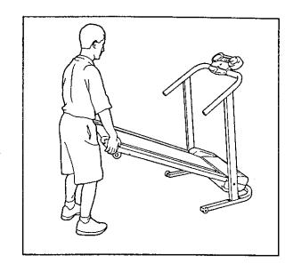
2. Move your right hand to the position shown and hold the treadmill firmly. Raise the treadmill until the latch pin is aligned with the hole in the handrail. Slide the latch pin into the hole. Make sure that the latch pin is inserted as far as possible into the hole. Lock the pin by pressing the end of the pin into the slot in the storage latch as shown in the inset drawing.
